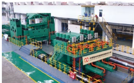
12,000t aerometal plank tension stretcher designed by SINO-HEAVYMACH
