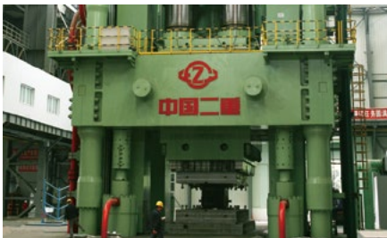
800MN forging press independently designed, manufactured and installed by CNEG
